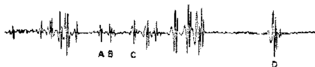
Figure 1. Typical Group of AE Events (After Chugh et al. 1972).
